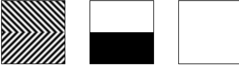
Figure 4.17: A textured image containing two differently textured regions with (u, v) = (0.05, 0.05) pixels -1 in the upper half and (u, v) = (0.05, -0.05) pixels -1 in the lower half (top), the channel assignment based segmentation using the complex approach (middle) and using the quaternionic approach (right). On this stage the quaternionic approach is apparently inferior. Its superiority will become obvious only in a later stage of the segmentation procedure.
