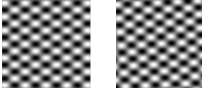
Figure 4.2: Two synthetic images. The second is a distorted version of the first one, where the distortion is the result of the affine transformation (A_1, \mathbf{b}_1) .
