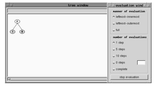
The first two steps of the execution consist in a substitution of the call F(1,0) and after that a simplification of the resulting expression as far as possible. They lead to an expression which is depicted on the tree window of KIEL as follows:
