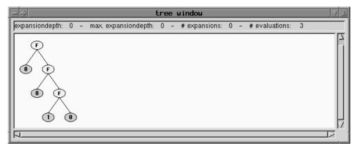
Already after these few steps it should be clear for a student how leftmost-innermost substitution works and that in the case of the expression F(1,0) its application leads to an infinite sequence of expressions, i.e., to "undefined" as result.
