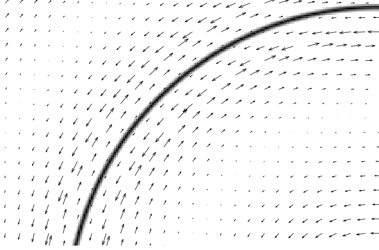
Figure 4: Monogenic phase of one part of fig. 3, left (curved line, displayed as underlying grayscale image). The phase is represented by the vector field which is obtained according to (14). Hence, the length indicates the rotation angle and the direction indicates the rotation axis. Note the phase-wrapping.
