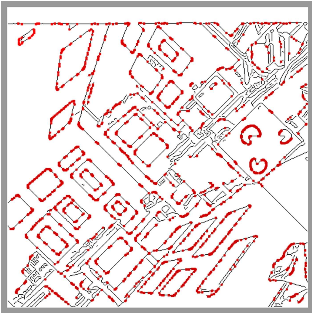
Figure A.4: All corners found in example image "lab", with confidence value \geq 0.99 and opening angle between 0 and 180 degrees.
