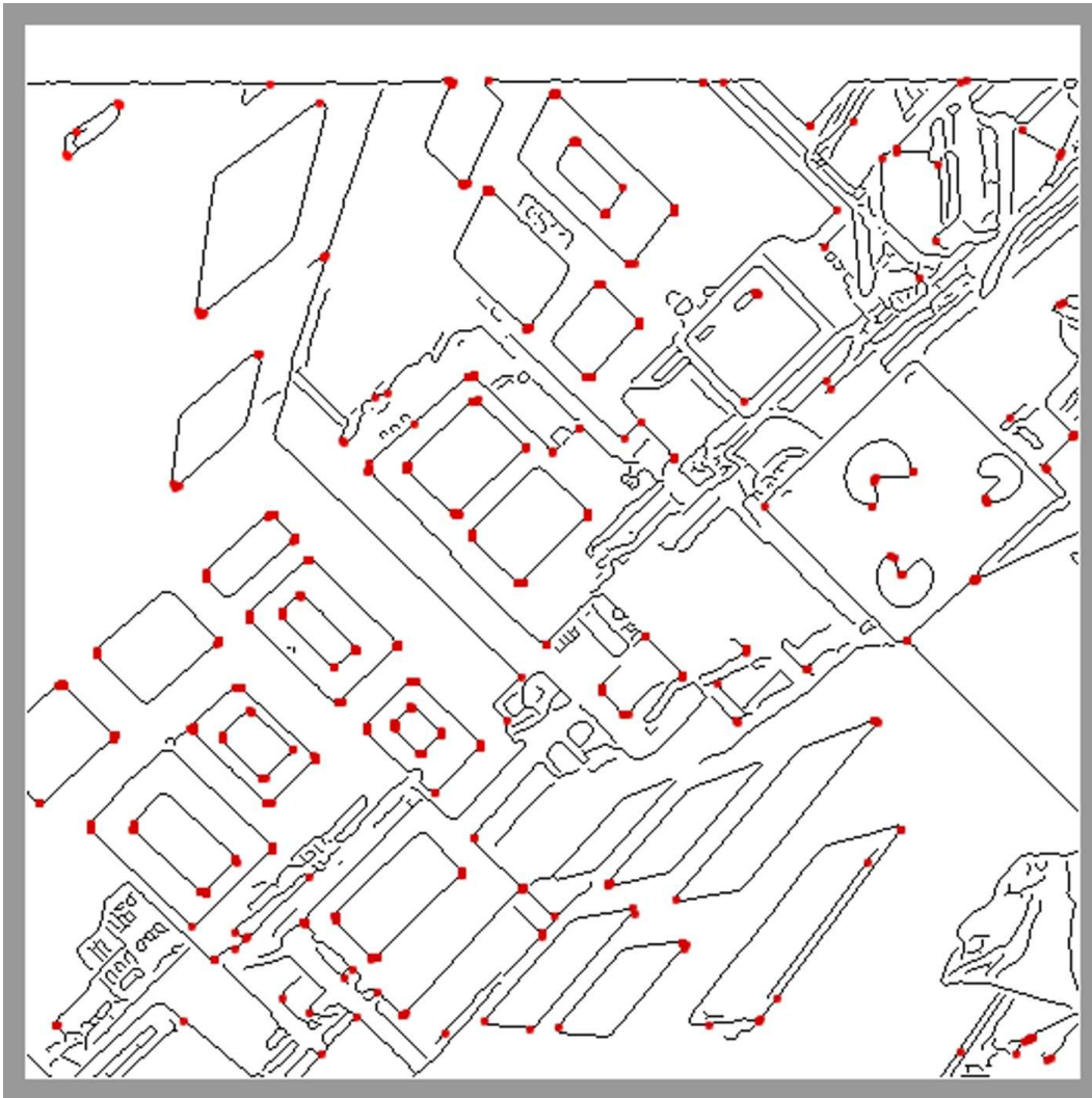
Figure A.6: All corners found in example image "lab", with confidence value \geq 0.99 and opening angle between 0 and 110 degrees.
