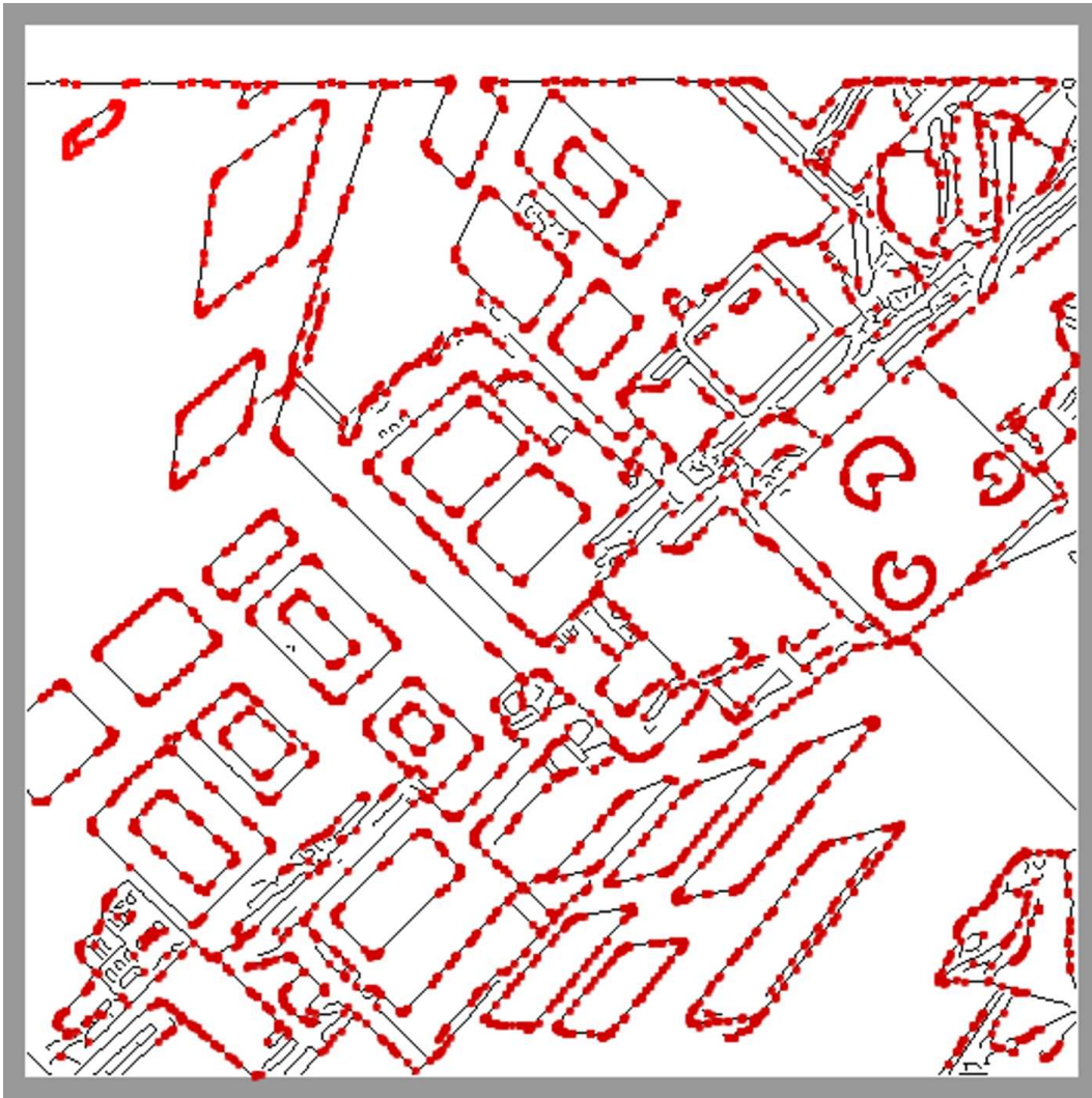
Figure A.3: All corners found in example image "lab", with confidence value \geq 0.50 and opening angle between 0 and 180 degrees.
