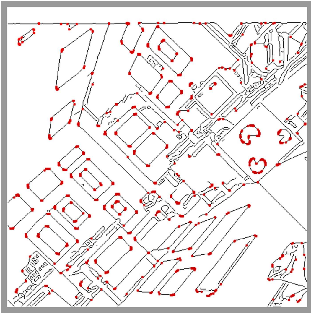
Figure A.5: All corners found in example image "lab", with confidence value \geq 0.99 and opening angle between 0 and 150 degrees.
