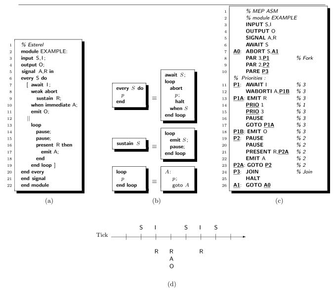
Figure 2: EXAMPLE: an Esterel module illustrating the parallel and preemption statements (a), the translation rules for the every, sustain and loop statements that are used when compiling the program (b), the resulting MEP assembler program (c), and a possible execution trace (d).
