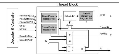
Figure 3: Architecture of the Thread Block
