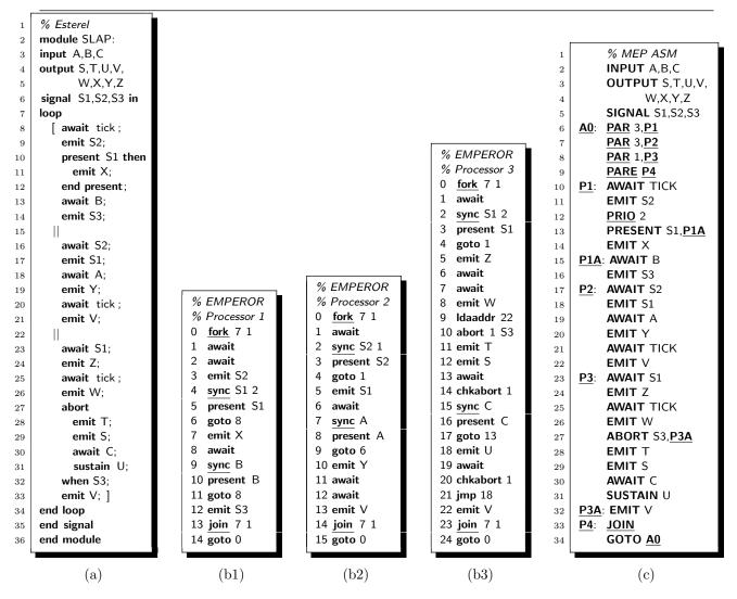
Figure 4: An Esterel module involving the parallel statement (a), and the corresponding assembler code for EMPEROR (b1/b2/b3) and for the MEP (c).
