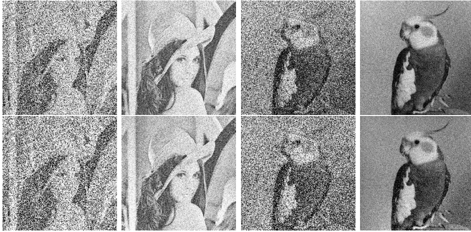
Fig. 6.6: Top row: noise contaminated original images. The first and third columns are images added with Gaussian additive noise (SNR=3). The second and fourth columns are images added with Gaussian additive noise (SNR=15). Bottom row: reconstructed results for the noise contaminated images.
