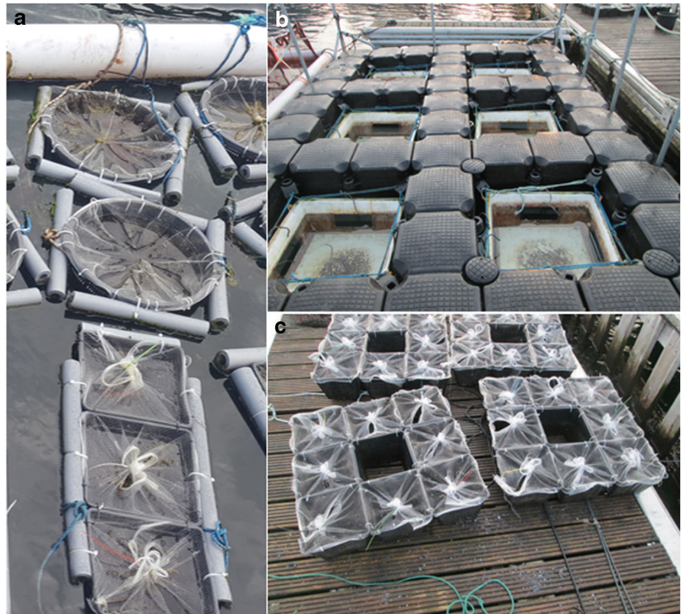
Fig. 1 a Package of cultivation baskets for experiment 1 (bottom, quadratic) and cultivation baskets for experiment 3 (top, round). b White boxes with side windows installed in the Jetfloat system. c Packages of cultivation baskets for experiment 2 which were inserted in the white boxes shown in b
