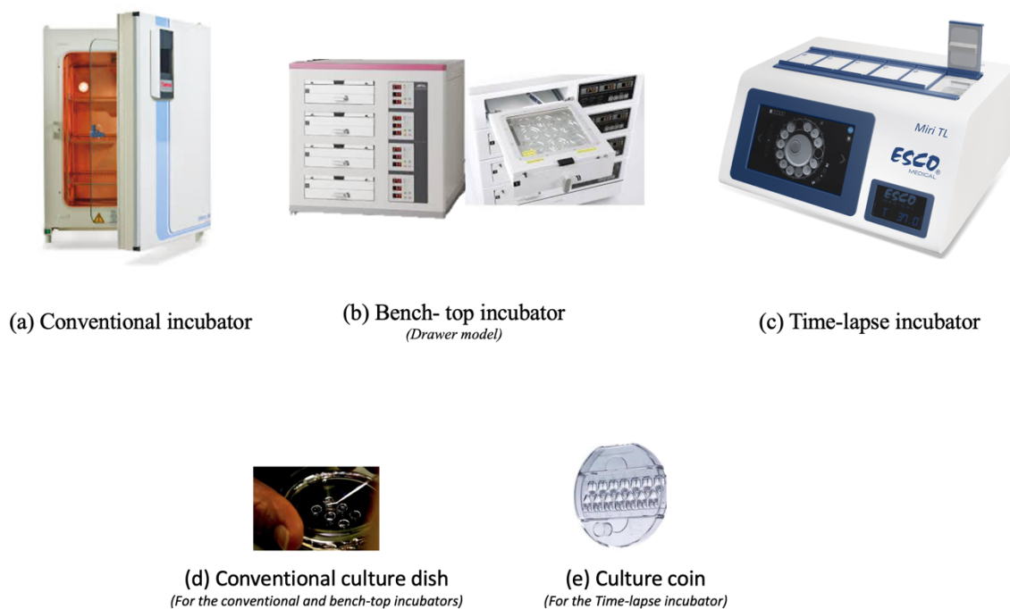
Figure 4: Different incubators and culture dishes used in the Lab. Incubators used for culture of embryos (a,b,c); Culture dishes used for culture of embryos in the incubators (d,e)
