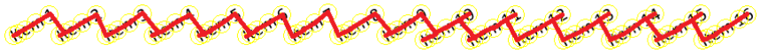
Figure 3.4. A block of rotated text with the corresponding MST on the center of mass of the characters to split the block into multiple text lines.
