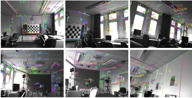
Figure 5.9. Six images taken from the sequence of the laboratory which includes 70 views and 165 lines. Those lines are shown in the images whenever they are detected.
