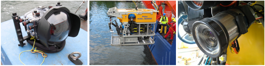
Figure 1.1. Left: SLR camera in underwater housing. Middle: ROV Kiel 6000 from Geomar Helmholtz center for Ocean Research. Right: deep sea flat port camera.
