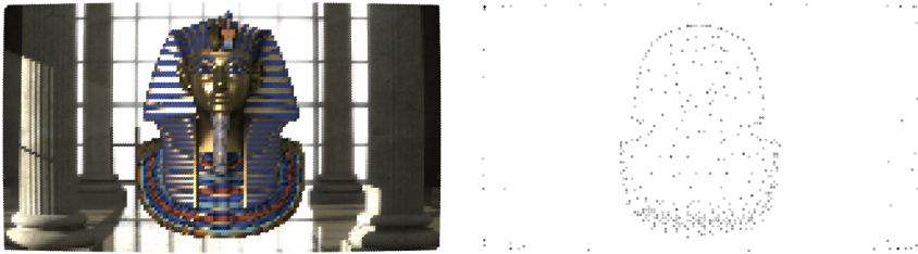
Figure 7.6. Simulated display overview with the viewpoint centred about 60 centimetres in front of the display (left) and position of the top ranking 393 viewpoints (right). The darker a viewpoint is coloured, the more important it is ranked.
