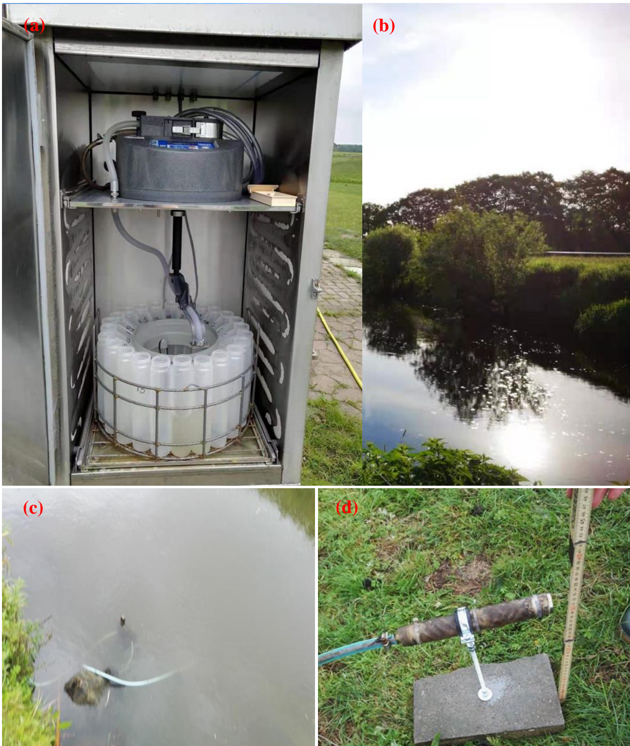
Figure 2-3. (a) ISCO sampler in Willenscharen, (b) sampling site of the river, (c) water tube collector installed in river, (d) view of the sampling probe.
