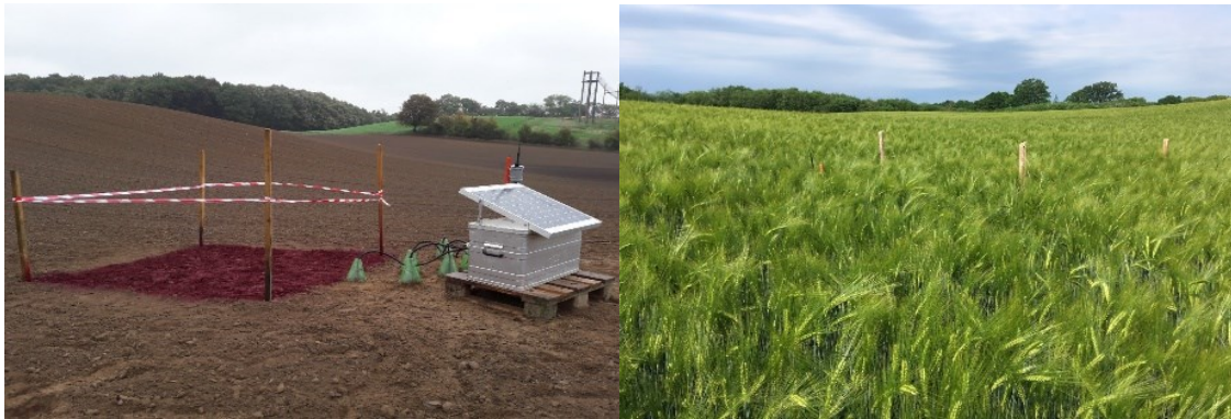
Fig 3-3: Left: Set up of tracer experiment at 4 m 2 plot equipped with six soil moisture sensors directly after pesticide and tracer application (10/01/2018) and right: winter barley at tracer site (06/06/2019).
