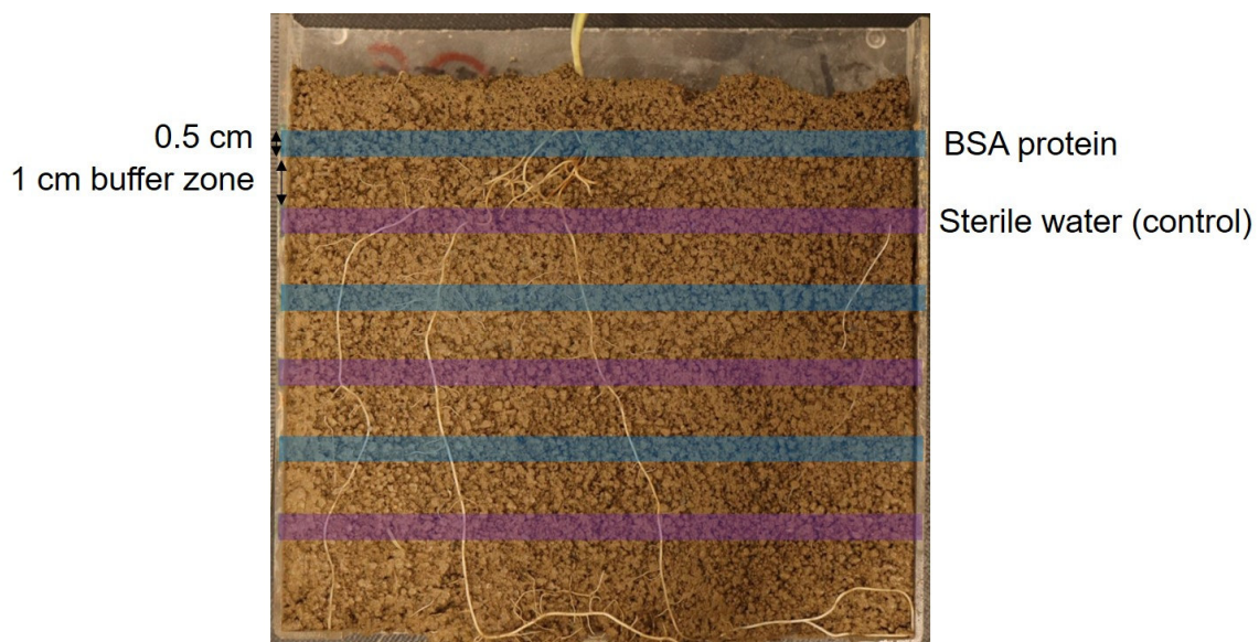
Figure 1. Rhizobox set-up showing the position of the protein and control (sterile water) horizontal bands in soil.
