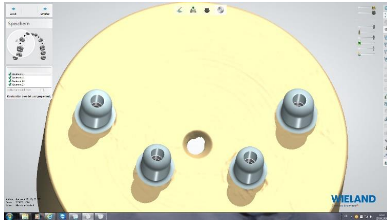
Figure 2. Designing of the abutments using the CAD-software.
