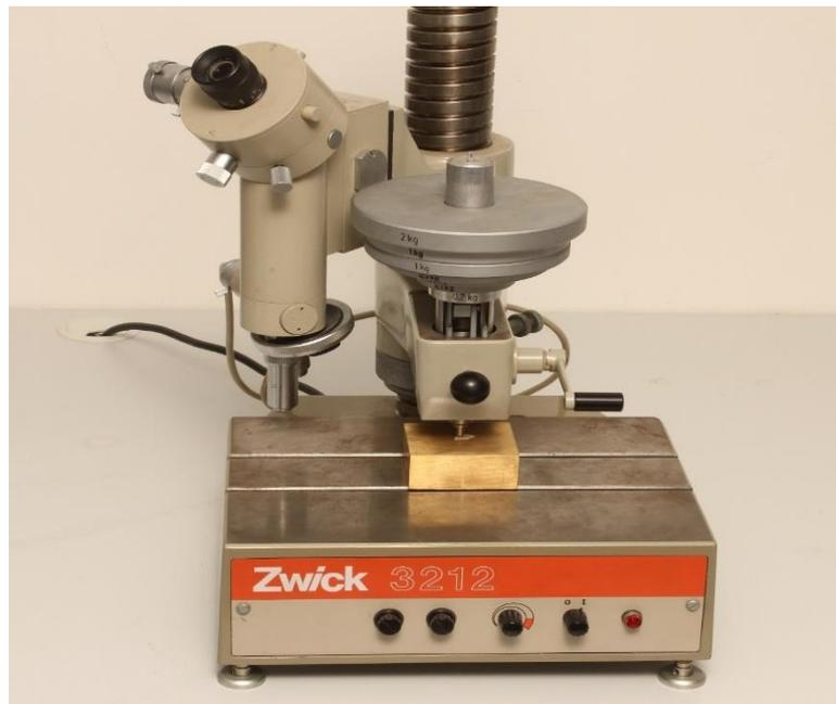
Figure 3: Vickers hardness testing machine
