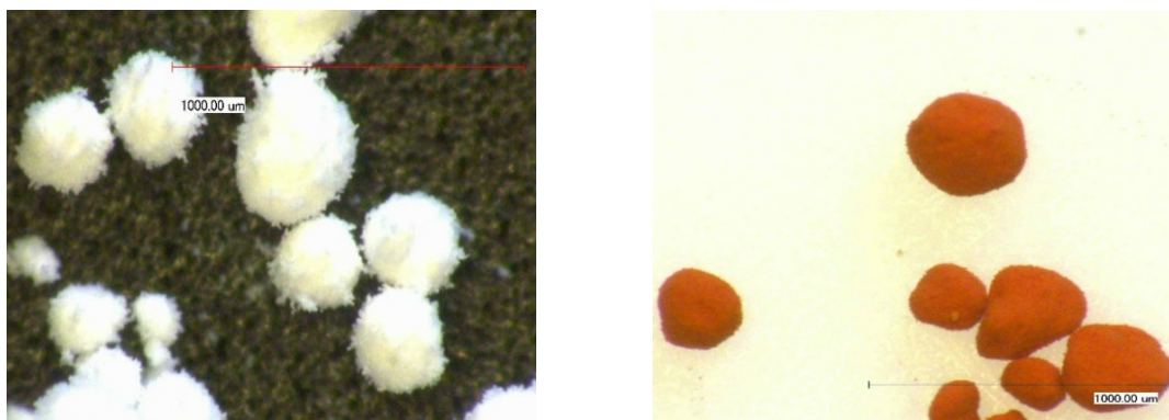
Figure 3.39: Softpellets consisting of ISN (left) and RIF (right), respectively. Images captured using digital microscopy with a magnification of 175x (adopted from Iwersen [142]).
