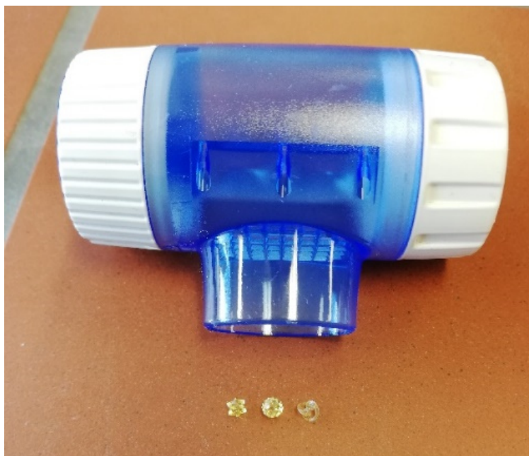
Figure 3.16: Image of the Twister ® device and the DAs with a diameter of 3 mm (from left to right: PC, SB and RK).
