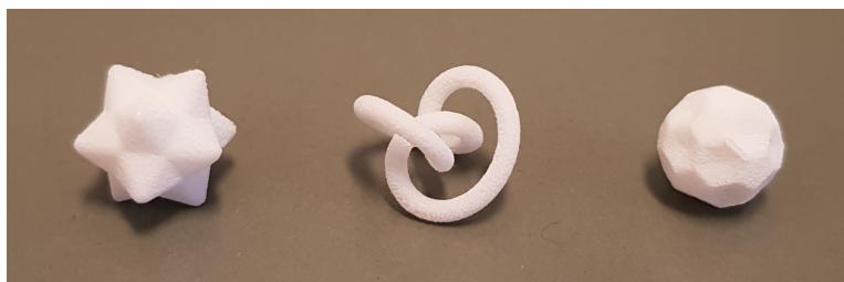
Figure 3.13: Additively manufactured geometries with 12 mm in diameter made by SLS printing (purchased from nobitec GmbH). From left to right: PC, RK and SB.
