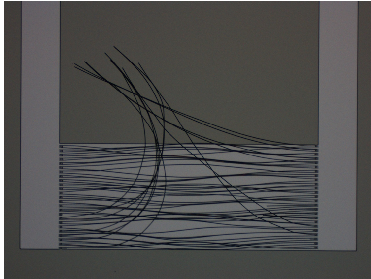
Figure 2.1: Light microscopy image of the photoresist AZ nLOF 2070 by MicroChemicals prepared for lift-off on ST-cut quartz. No HMDS was applied and therefore the photoresist delaminated.
