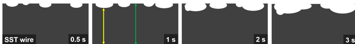
Figure 5.3: Schematic illustration of bowl-like structure formation at the constant current application of 2 A (4 A/cm 2 ) with increasing sculpturing time using 0.25 M HCl-based electrolyte and showing the nominal SST wire thickness (green arrow) and the effective thickness (yellow arrow).
