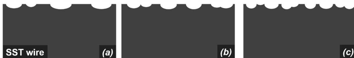
Figure 5.4: Schematic illustration of bowl-like structure formation at the current pulsing application of 2 A (4 A/cm 2 ) using 0.25 M HCl based electrolyte and 1 s total sculpturing time; (a) One anodic current spike (constant current application), (b) Two anodic regimes current spikes (TPS) and (c) Multiple anodic current spikes (MPS).
