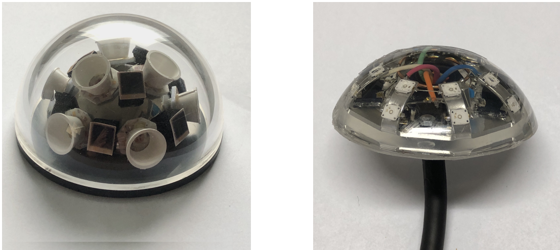
Figure 4.32: Left: Model of transducer utilizing a 100 mm dome port and comprising 9 pcs. large area PD and 9 LED elements. Right: Pressure-neutral potted transmitter head of 95 mm diameter, including 4 segments of each 4 power LEDs and driver circuits.
