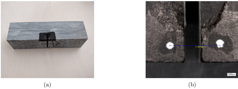
Figure 5.14: The application of image processing technique with (a) the predefined reference points for measuring the CMOD, and (b) the measured rough distance using an optical microscope (Sattari et al. 2021)
