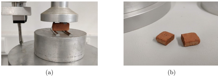
Figure 5.2: The brick under three-point bending test (a) before, and (b) after failure
