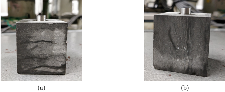
Figure 5.32: The fracturing paths through the Opalinus clay (a) 1 st stress configuration, and (b) 2 nd stress configuration (Vowinckel et al. 2021)
