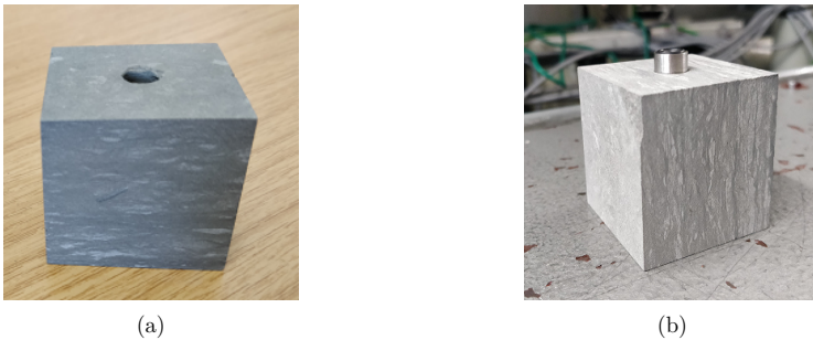
Figure 5.31: The orientation of the embedded layers (a) perpendicular, and (b) parallel to the direction of the borehole pressure configuration (Vowinckel et al. 2021)
