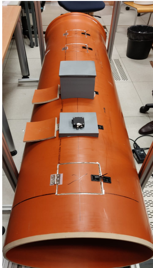
Figure 2.4: The transmission channel in the form of a tube-like structure with multiple flaps over a maximum length of 2.38 m, where the detection modules can be mounted.
