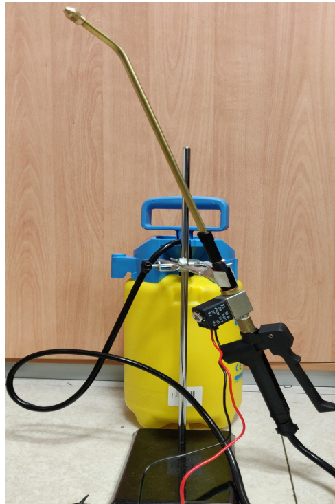
Figure 2.1: Solenoid valve operated Gloria 3 pressure sprayer as the transmitter with water-based solution of the information carrier.
