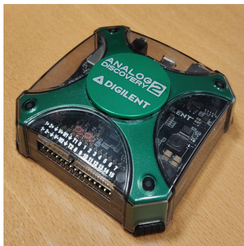
Figure 2.2: A micro-controller device Analog Discovery 2 facilitating the opening and shutting mechanisms of the solenoid valve.
