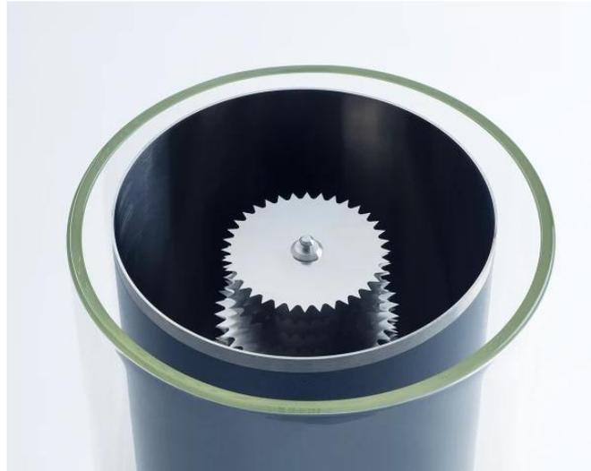
*Figure 6.10: Particle collector of the Büchi Nano Spray Dryer B-90 comprising the cylindrical shaped collecting electrode in the centre of which a pile of star-shaped foils is located. The particles are intended to attach to the inner surface of the cylindrical shaped collecting electrode [79].*
