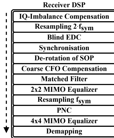
Figure 2.7: DSP chain for coherent PolMux transmission used in this work; EDC: electrical dispersion compensation; SOP: state of polarization; CFO: carrier frequency offset; PNC: phase noise compensation; MIMO: multiple input multiple output.
