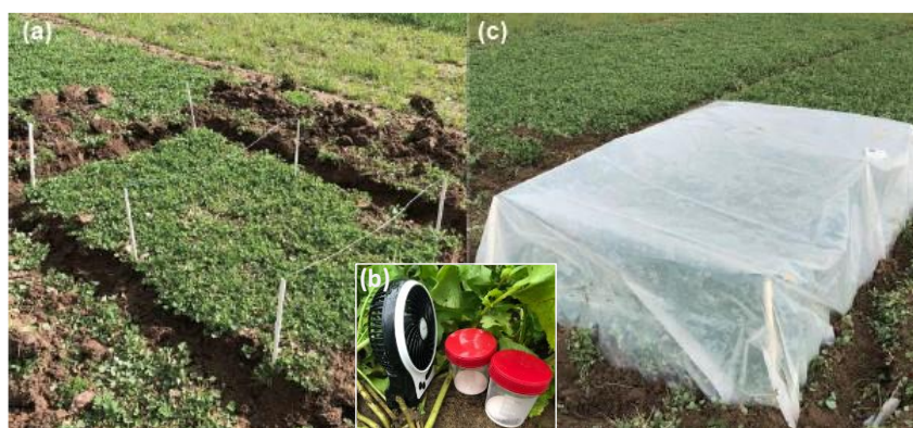
Figure 4 ^{13}\text{C} pulse labeling of cover crops. (a) Preparation of the labeling area; (b) Placement of \text{NaH}^{13}\text{CO}_3 in the chamber; (c) Sealed chamber with temperature monitoring.
