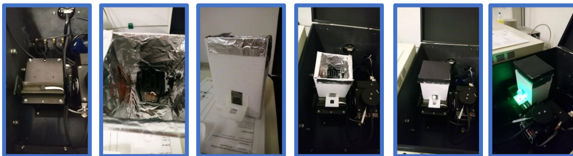
Figure SVIII.1: Setup for irradiation with CPL inside the CD spectrometer for determination of ellipticity \theta depending from the irradiation time.
