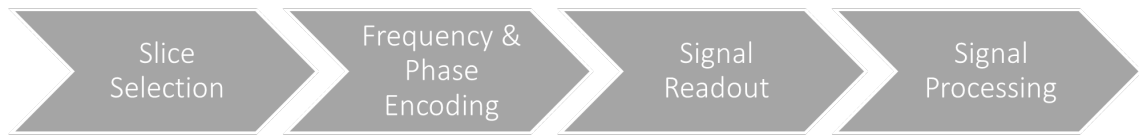
Figure 4.7: The image formation process in MRI begins with selecting a slice from the volume of interest. To capture elements of this slice, frequency and phase encoding occurs prior to a signal readout. The signals are then processed to form the final image.
