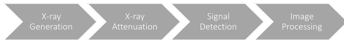
Figure 4.2: A scanning procedure typically consists of x-ray generation, where then after the x-rays are attenuated by the subject. The x-rays which pass through the subject are then detected and converted into signals which are further processed into a final image.
