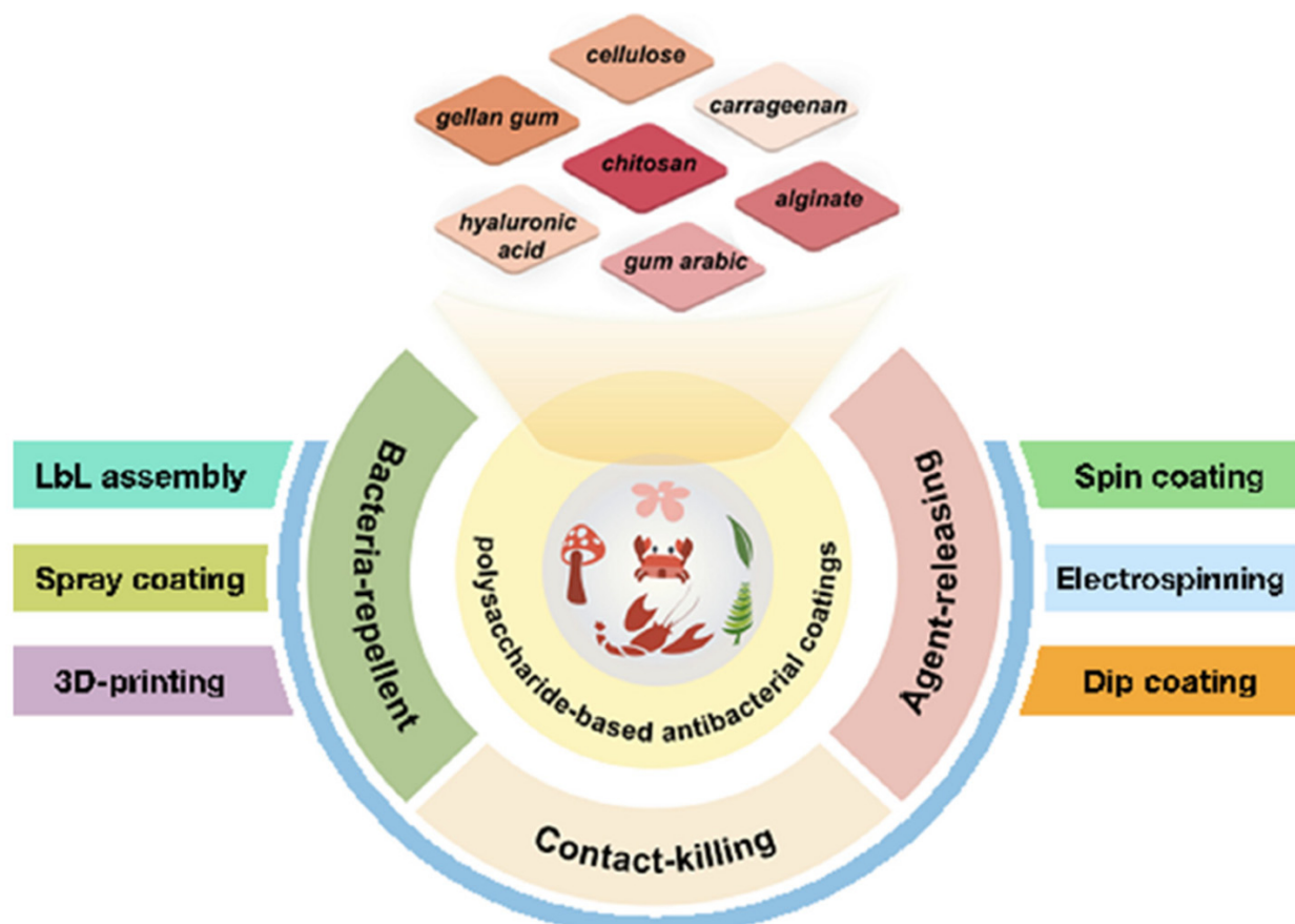
Figure 9. Illustration of polysaccharide-based antibacterial coating technologies: main types of polysaccharides, strategies for killing bacteria, and typical fabrication methods [74].
