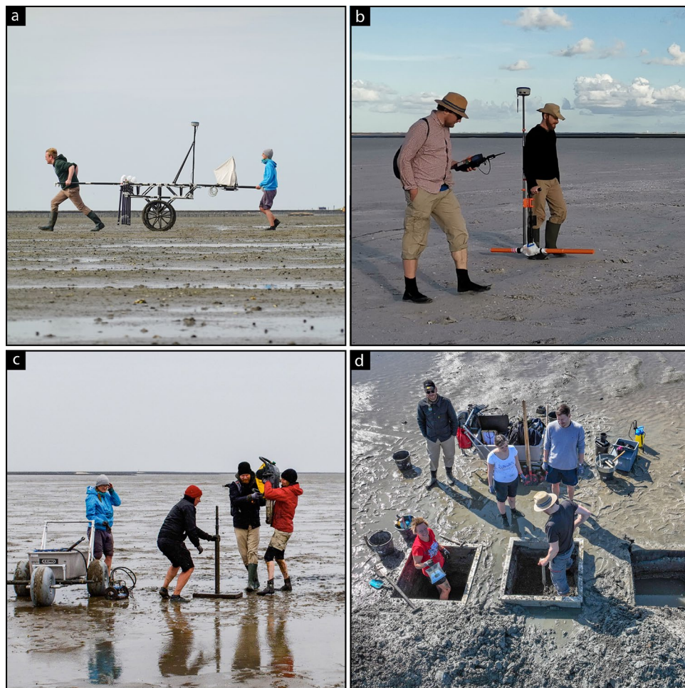
Figure 7. Methodological approach. (a) Magnetic gradiometry in the tidal flats during low tide (Photo: F. Schlütz, Kiel). (b) EMI prospection of sites selected from magnetic gradiometry results 45 . (c) Coring at specific sites selected from geophysical prospection results (Photo: J. Lemm, Berlin). (d) Test pit excavations to obtain soil profiles for characterization of sedimentary units and identification of potential archaeological structures. Informed consent was obtained from all subjects and/or their legal guardian(s) for publication of identifying information/images.
