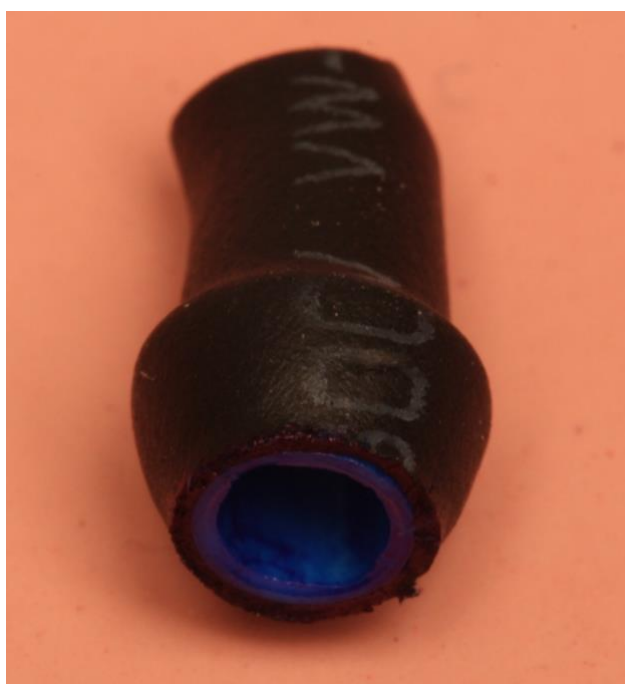
Figure 7: Stained intaglio surface of zirconia abutments.
